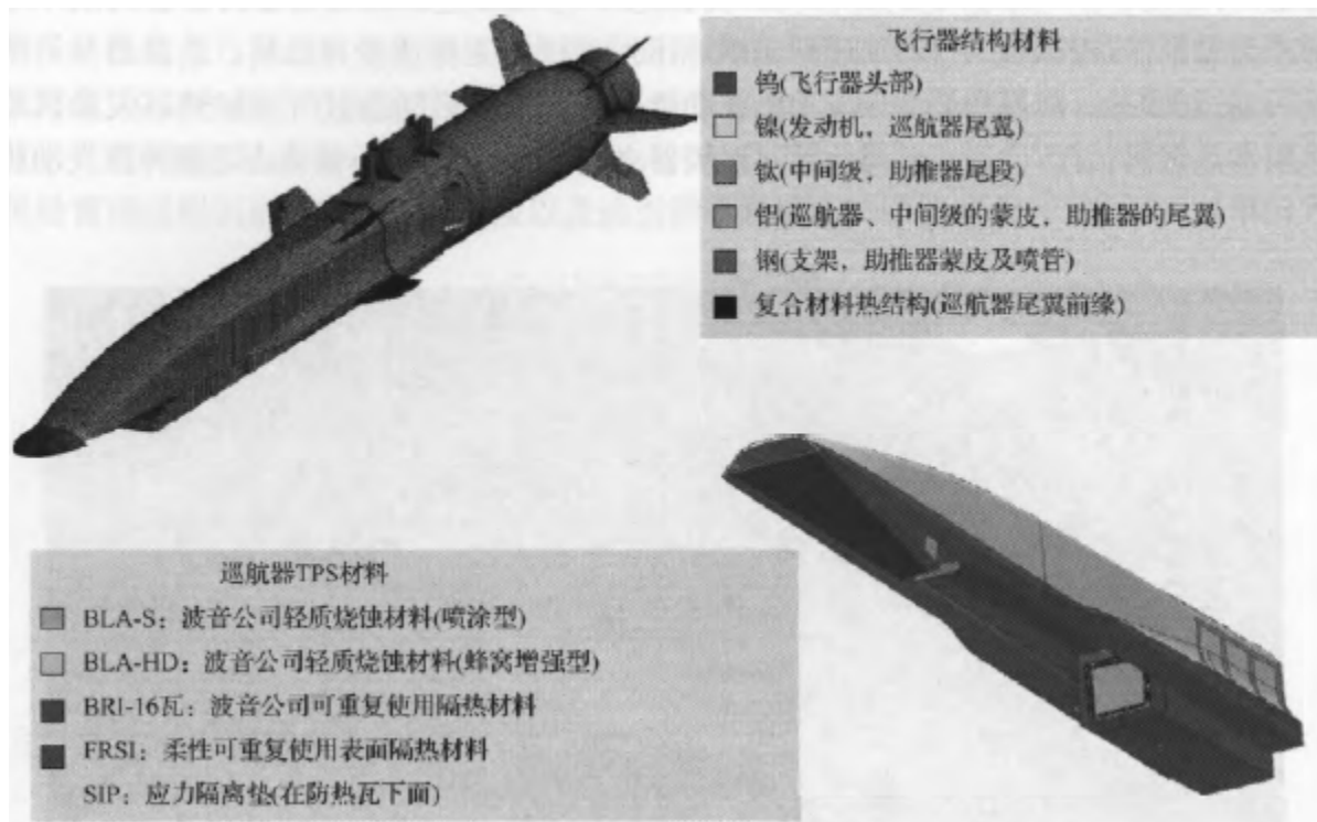
Figure 9-37: X-51A Structure and Thermal Protection Materials
