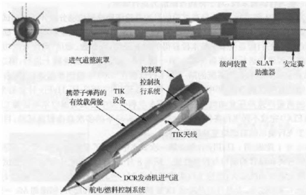
Figure 9-27: Schematic diagram of the HyFly aircraft
