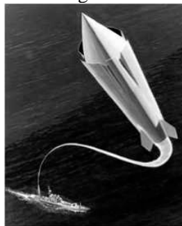
Figure 1-8: Schematic diagram of the ship-launched HyFly hypersonic missile
