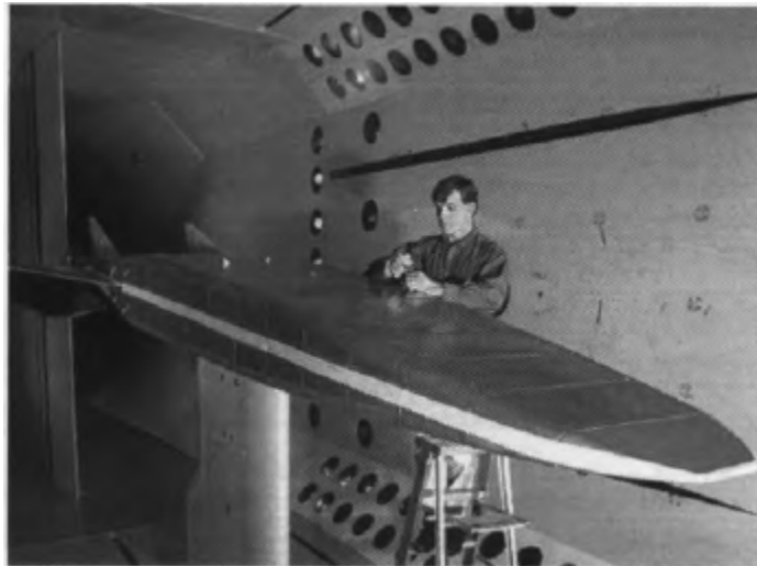
Figure 9-5: Model of the X-30 test vehicle in a wind tunnel
