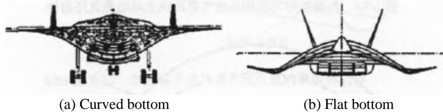
Figure 5-86: Front view of an arc-shaped and flat-bottomed waverider aircraft
