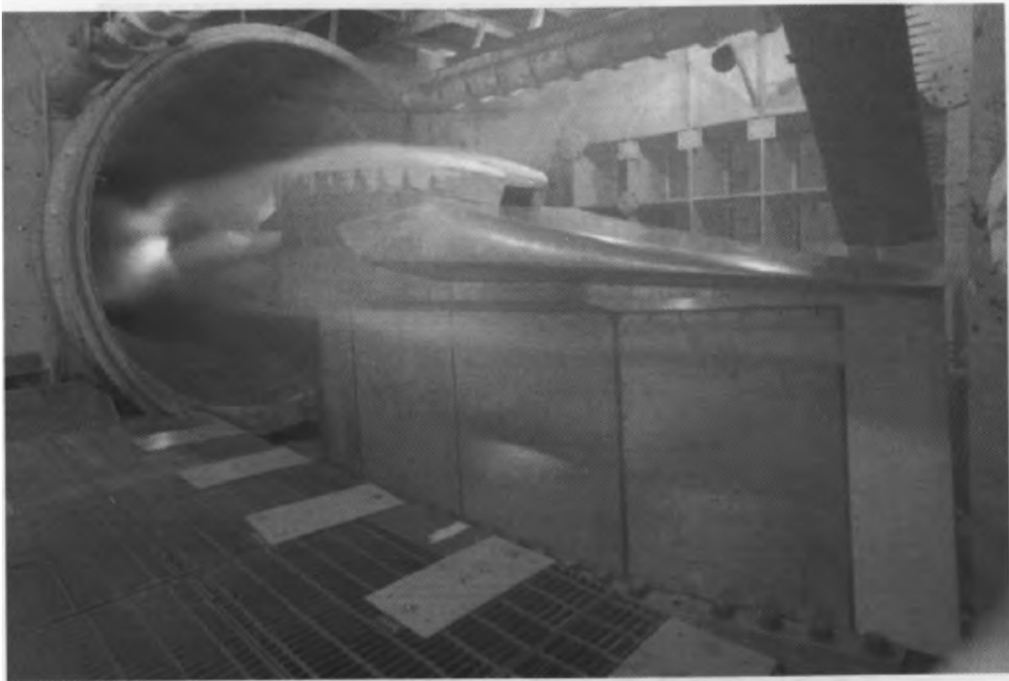
Figure 9-43: GDE-2 engine in a NASA-LaRC 8 ft wind tunnel
