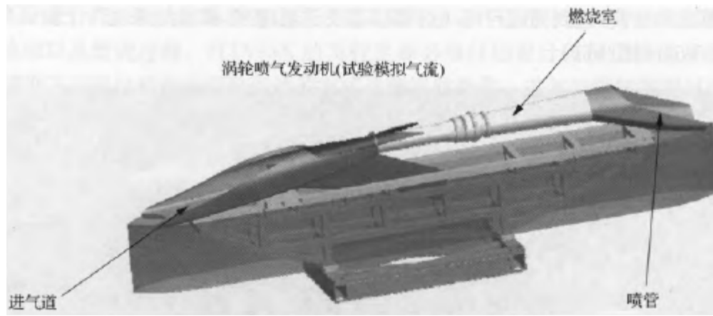
Figure 9-56: FaCET free-jet engine model with support bench
