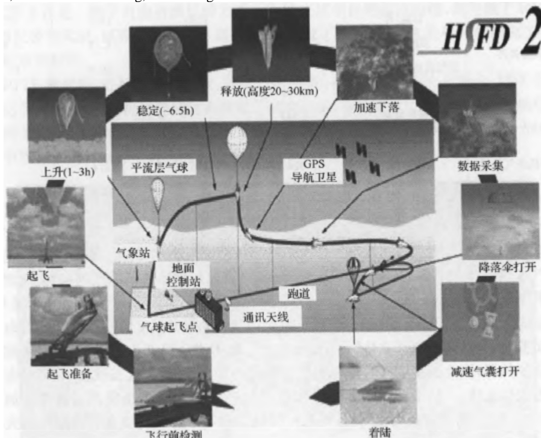
Figure 13-10: HSF2 flight test procedure
