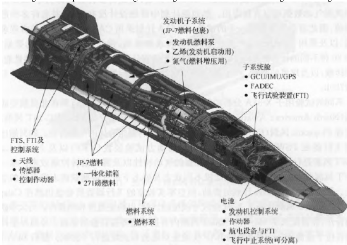
Figure 9-38: X-51A subsystem composition
